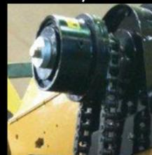
Heavy duty auto clutch eliminates shear pins (tested over 1500 times without failure)
