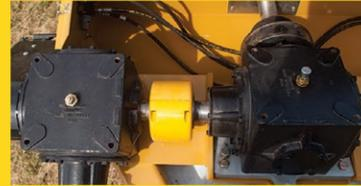
Two 330 pound gear boxes with 2 3/4 inch output shafts
