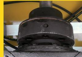
Guardian rubber dampeners between gear box and impeller shaft
