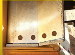
Durable carbon steel wear edges on impeller paddles
