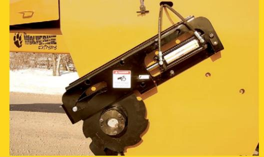
Super heavy duty hydraulic reverser (reverses kicker shaft to clear soil for easy restart)
