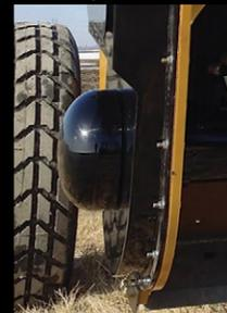
Oil bath chaincase is narrower to reduce drag in soil
